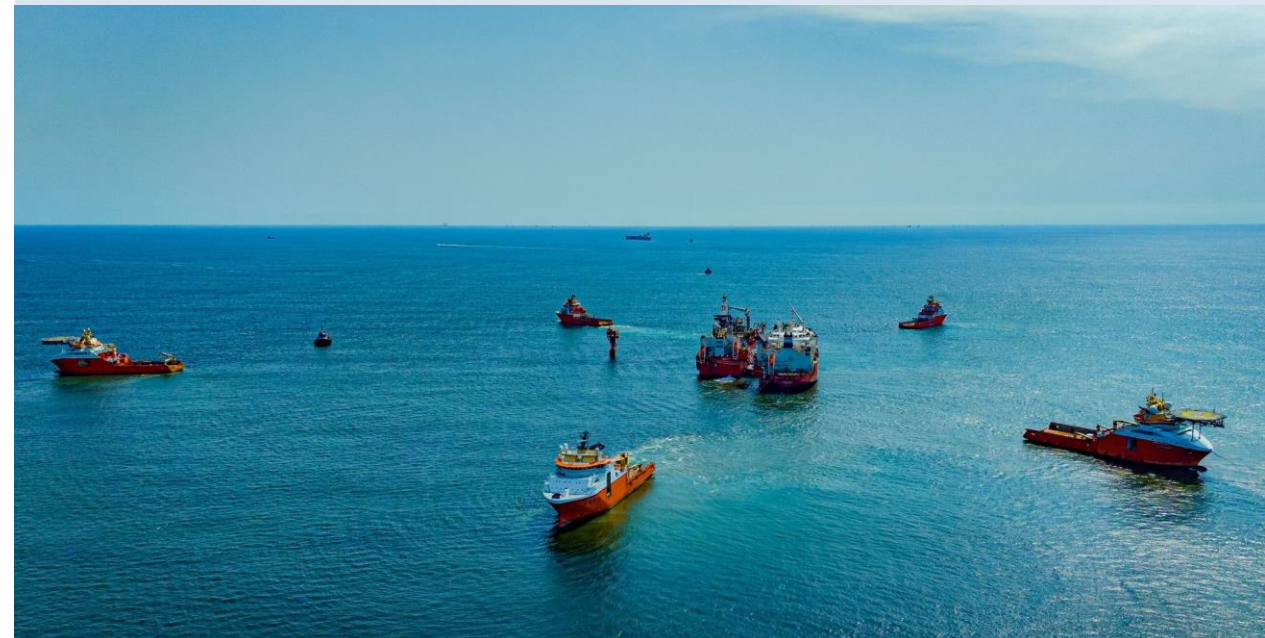
5 of the groups AHTS vessels were in Q4 23 involved in anchor installation and hook up of floating units in Congo
